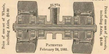
All rolling parts of the above wheels and journals are of steel, case hardened, each truck consisting of 36 rolls, 1/4 inch in diameter, making a total of 1/4 rolls to a set. Testimonials as to the speed and durability of this Bearing have been received from the leading skaters. This bearing can be applied to the BARNEY & BERRY Skates only.
